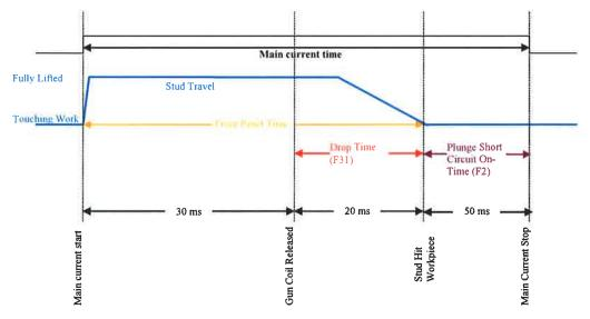
The resulting Actual Weld Time is 50 ms. The main current would be on for the Front Panel Time + Plunge short circuit on-time (F2) = 50ms+50ms=100ms, but the arc would exist only during the Actual Weld Time, or 50ms.
