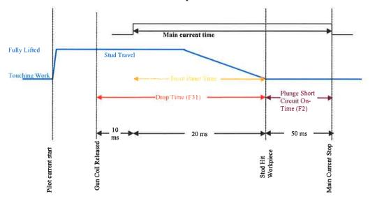
The resulting Actual Weld Time is 20ms. The stud would still take 30ms to drop, but the main current and main arc would only be 20ms.
