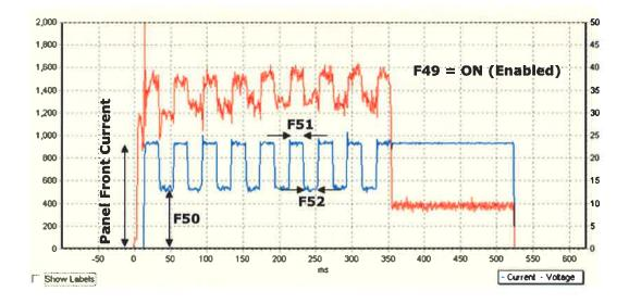
Due to low circuit inductance, it is possible to see current regulation errors when the pulse low current is too low, or the gap between high and low levels is too big. By default pulse main arc current is disabled.
